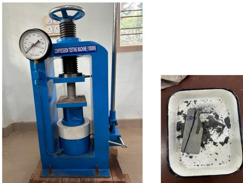
Fig. 4: Compressive testing machine
