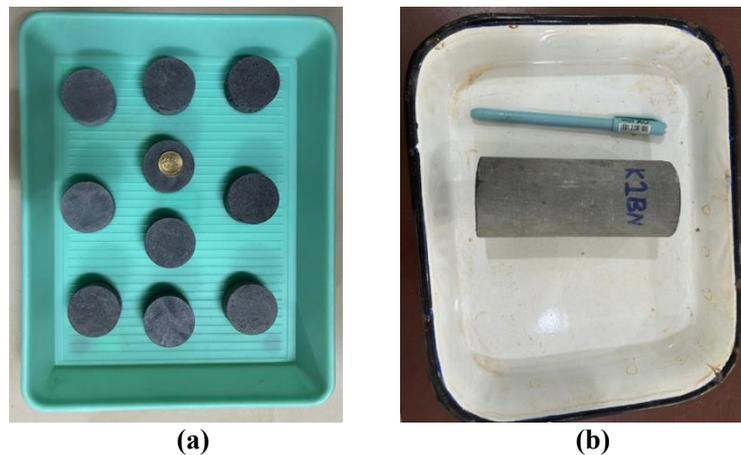
**Fig. 1: Rock sample photos for testing, (a) Disc sample for thermal conductivity test and (b) Cylindrical samples for P-wave velocity and UCS testing**
