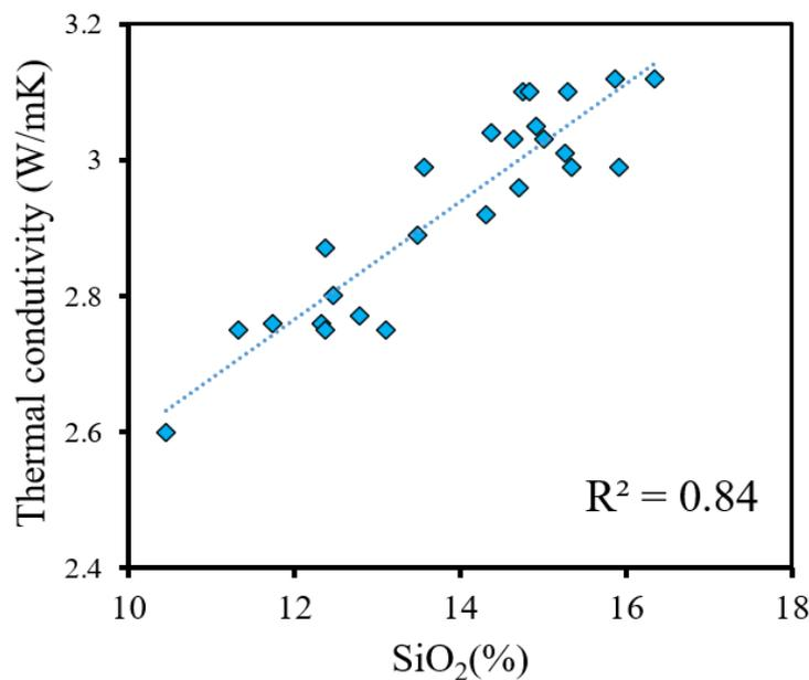
**Fig. 7: TC versus SiO<sub>2</sub>(%)**
