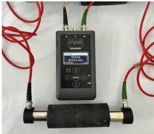
Fig. 3: Measuring the velocity of P-waves in rocks.
